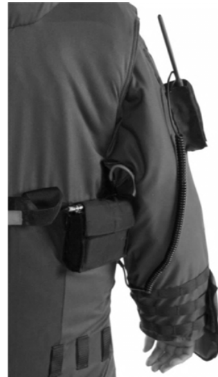
The power supply is provided in a pouch which is worn on the right hand side of the suit.
