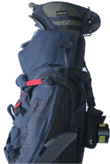
The PAPR air filtration system is mounted on the rear of the smock. The hoses are integrated through the rear of the collar to mate with the NBC mask underneath the helmet.
