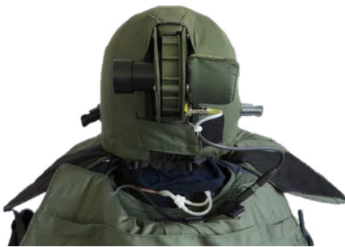
The harness cable will provide power to the helmet fan & communications
